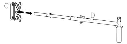
STEP3- Remove pin on B and insert into D top of opening and adjust to desired length. Then install pin.
