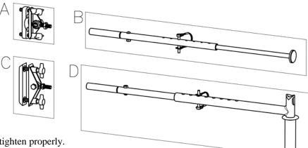
**STEP1**- Insert **A** Into **B** and screw in and tighten properly.
