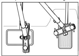
3. You should be able to slide the brake mount over the pedal in a vertical placement. Then tighten finger screws evenly and verify that the clamps are secure. Be sure that the AZ-1 portable hand control system doesn't interfere with anything that would compromise safety. If the AZ-1 cannot be adjusted to the proper length contact the company where you purchased and return for replacement
